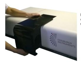
Pull the sample module out to the front, using the gap on the bottom between the sample module and the FS5 enclosure.
