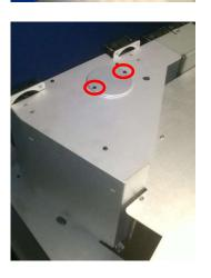
FS5 and the Y adjustment on the bottom left of the instrument.
